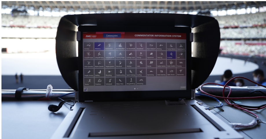
Figure 4 Commentator Information System (CIS) which provides broadcasters with results and statistics from the field as well as background information on athletes
