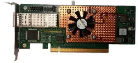
Figure 2: BXI V2 Standard PCI card
