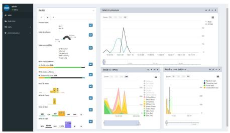
Bull IO Instrumentation has been developed as a highly scalable application to minimize the impact of collecting samples of its metrics. It is implementing a hierarchical 2 levels MongoDB database.
