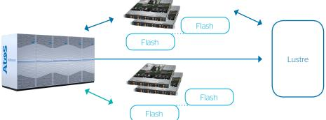
With Bull Smart Burst Buffer, transparent caching will rely on I/O calls interception through the scheme implemented in the Bull IO Instrumentation library.
