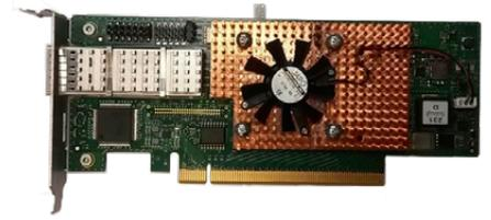
Figure 2: BXI standard PCI card
