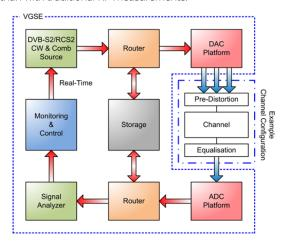
The VGSE is a generic wide-band waveform and traffic generator and analyzer working in a closed-loop mode for end-to-end system validation and optimization. It supports CW, modulated-only, and DVB-S2/RCS2 carriers at bandwidths up to 500 MHz.
